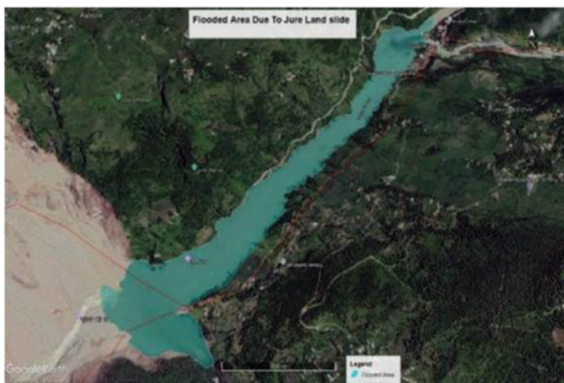
Figure 6 Participatory GIS-based delineation of the flooded area in Jure caused by the landslide-induced blockage of the Sun Koshi River.
